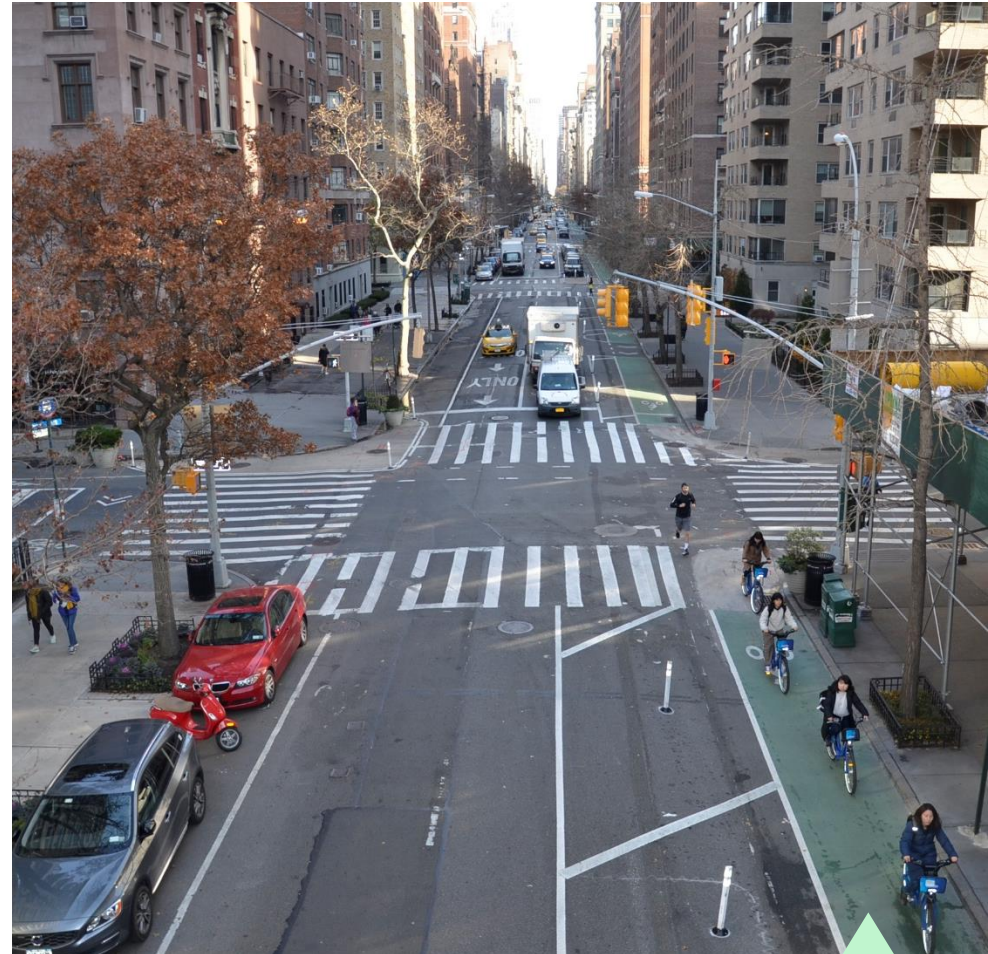
2017 upgrades included a bike lane to Protected Bike Lane conversion on 5 th Avenue in Manhattan, featuring both Mixing Zones and Fully Split Phase (shown) intersections
